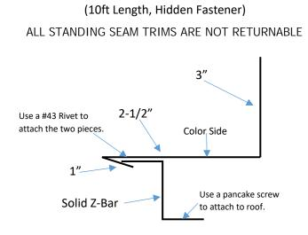
Standing Seam End/Head Wall Flashing w/Solid J-Channel
