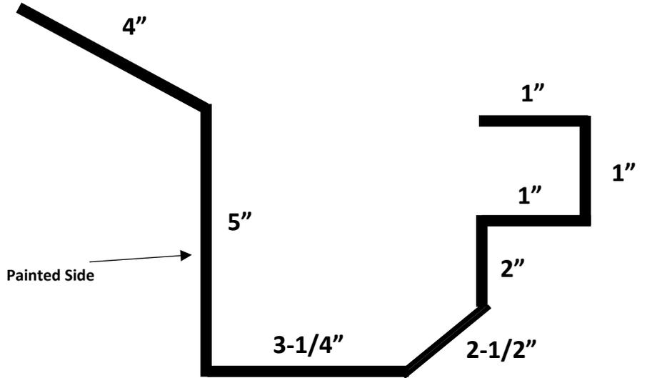
Does not include Ends, you will need to fabricate your own ends using a hand bender.
