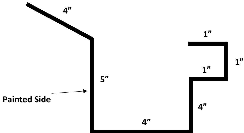
Does not include Ends, you will need to fabricate your own ends using a hand bender.
